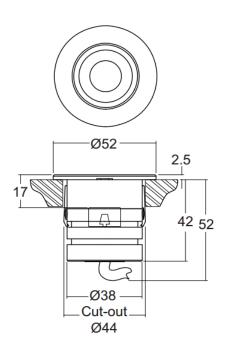
**/SC - Spring clip fixing**Useful for plinth or downlight applications
