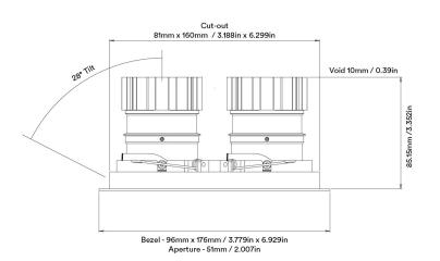
Unit height increases by 21.65mm / 0.85in for Spot and Elliptical beams.
