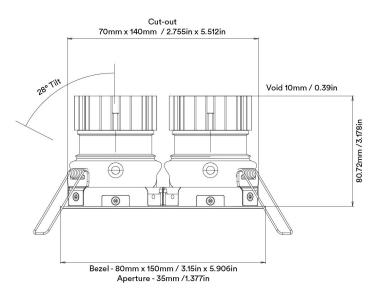
Unit height increases by 21.65mm / 0.85in for Spot and Elliptical beams.
