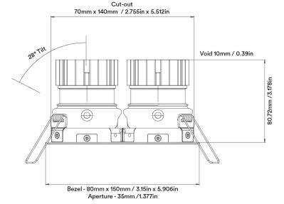
Unit height increases by  $21.65 \, \text{mm} / 0.85 \, \text{in}$  for Spot and Elliptical beams.
