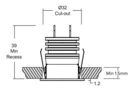
LED and optic position recessed by 10mm for reduced glare.
