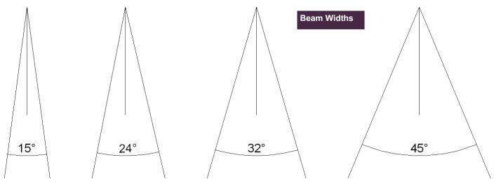
Varying your selected beam width can be very effective, for example: using a very narrow beam (c.8-15 degrees) to uplight a column or using a wide beam to create broad pools of soft light in living areas.
