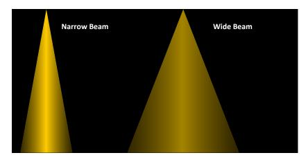
By selecting different beam widths for fittings you control the spread and dispersion of light.
